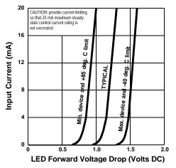
Figure 3. Input Characteristics (Current Controlled)
